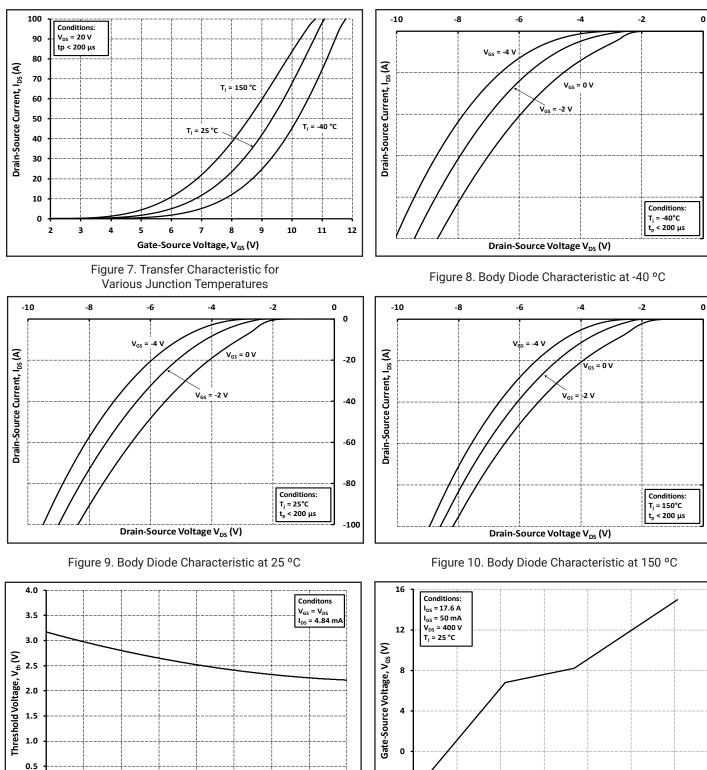
Figure 11. Threshold Voltage vs. Temperature
