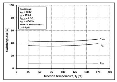
Figure 25. Clamped Inductive Switching Energy vs. Temperature
