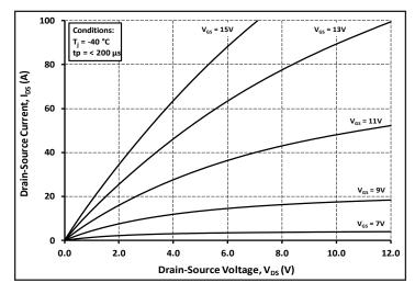
Figure 1. Output Characteristics T<sub>J</sub> = -40 °C
