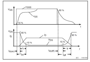
Figure 27. Switching Times Definition
