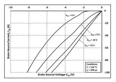
Figure 15. 3rd Quadrant Characteristic at 150 °C
