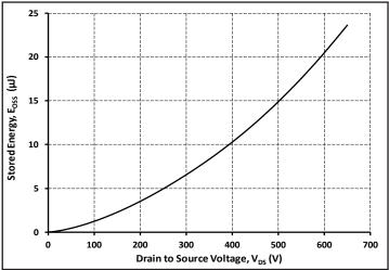
Figure 16. Output Capacitor Stored Energy
