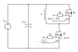
Figure 28. Clamped Inductive Switching Waveform Test Circuit
