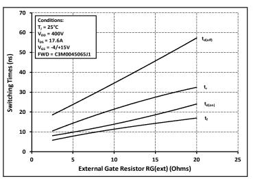
Figure 26. Switching Times vs  $R_{G(ext)}$
