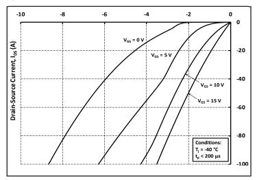
Figure 13. 3rd Quadrant Characteristic at -40 °C
