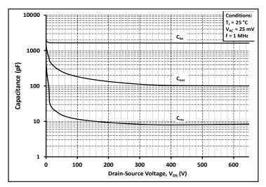
Figure 18. Capacitances vs. Drain-Source Voltage (0 - 600V)
