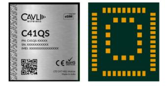
C41QS is an Cat NB2 Module compatible with 3GPP E-UTRA Release 14 standards supporting frequency bands B1/B2/B3/B4/B5/B8/B12/B13/B14/B17/B18/ B19/B20/B25/ B26/B28/B66/B70/B85 making it usable globally while consuming very low power. The module comes in a compact form-factor of 17.7mm x 15.8mm x 2.0mm ideal for size constrained applications. The module supports an optional integrated GNSS, and eSIM enabling Global Connectivity and Device management features powered by Cavli Hubble platform.
