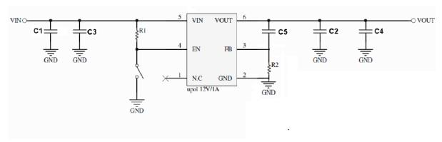
FIG.27 REFERENCE CIRCUIT FOR GENERAL APPLICATION
