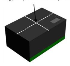
FIG 29. Case Temperature Sensing Point
