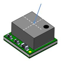
FIG. 29 Case Temperature Sensing Point
