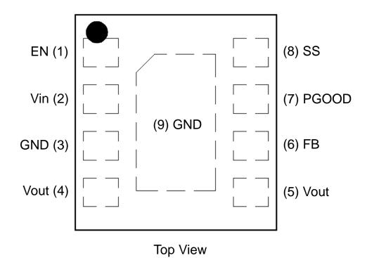
Fig.3 Pin configuration
