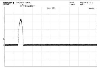
**Figure 7:** Output over voltage protection at 110/220Vac,21A lout, VOUT:5V/div, 500mS/div
