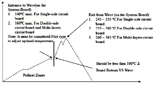
Note: The temperature is measured on solder joint of pins of power module.
