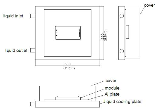
Figure 12: Thermal test setup
