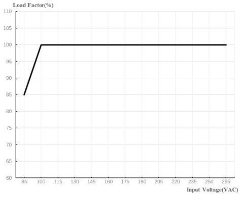
Figure 11: Input voltage derating curve
