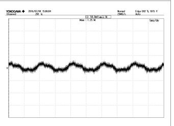
**Figure 5:** Vout start up with Enable on at 220Vac,21A lout, TOP:Vout, 10V/div, 500mS/div BOTTOM: Vin, 500V/div, 500mS/div
