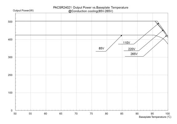
Figure 14: Thermal derating curves
