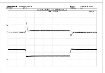
**Figure 3:** Output voltage vs. Output current @ Vin=110/220VAC
