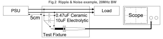
Fig. 3 Ripple & Noise measurement circuit
