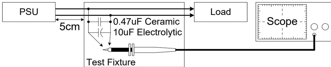
Figure 5 Ripple & Noise testing set up
