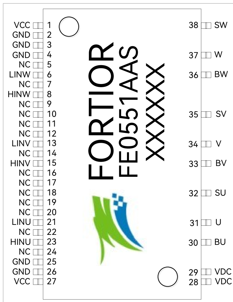
Figure 1-3 FE0551AAS SSOP A54-38 Pinout Diagram
