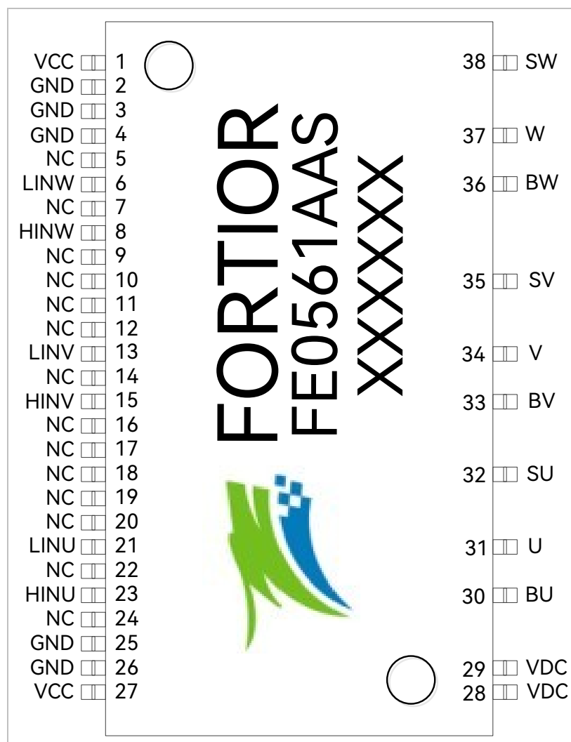
Figure 1-3 FE0561AAS SSOP A54-38 Pinout Diagram
