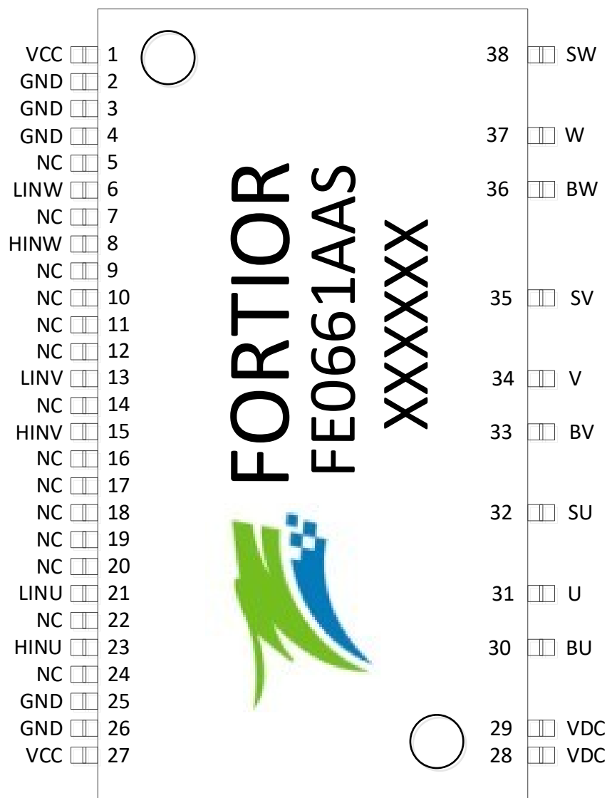
Figure 1-3 FE0661AAS SSOP A54-38 Pinout Diagram
