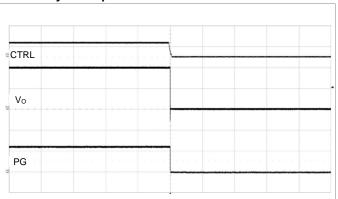
Output disabled by CTRL pin.  $V_1$  = 12 V,  $I_0$  = 80 A. Scale from top: 5, 0.5, 2 V/div, 20 ms/div.
