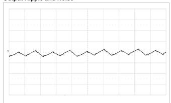
Fundamental output voltage ripple at V<sub>I</sub> = 12 V, I<sub>O</sub> = 60 A, C<sub>OUT</sub> = 8 x 330  $\mu$ F/10 m $\Omega$  + 20 x 100  $\mu$ F Scale: 10 mV/div, 1  $\mu$ s/div, 20 MHz bandwidth. See section Output Ripple and Noise.
