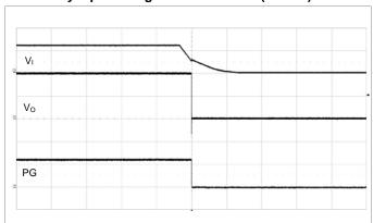
Output disabled by removing V<sub>I</sub>.  $V_I$  = 12 V,  $I_O$  = 80 A. Scale from top: 10, 0.5, 2 V/div, 20 ms/div.
