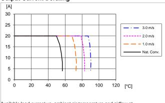
Available load current vs. ambient air temperature and airflow at  $V_{\rm I}$  = 12 V.
