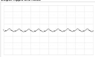
Fundamental output voltage ripple at V<sub>I</sub> = 12 V, I<sub>O</sub> = 20 A, C<sub>OUT</sub> = 4 x 330 µF/10 m $\Omega$  + 10 x 100 µF Scale: 10 mV/div, 2 µs/div, 20 MHz bandwidth. See section Output Ripple and Noise.
