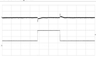
Output voltage response to load current step change (25%–75%–25%) at  $V_{\rm l}$  = 12 V,  $C_{\rm OUT}$  = 4 x 330  $\mu F/10$  m $\Omega$  + 10 x 100  $\mu F,$  di/dt = 2 A/ $\mu s,$  ACSR Gian=219 and ASCR Residual=82. Scale from top: 50 mV/div, 10 A/div, 500  $\mu s/div.$
