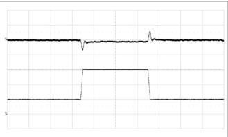
Output voltage response to load current step change (25%–75%–25%) at V<sub>I</sub> = 12 V, C<sub>OUT</sub> = 8 x 330  $\mu$ F/10 m $\Omega$  + 20 x 100  $\mu$ F, di/dt = 2 A/ $\mu$ s, ACSR Gian=219 and ASCR Residual=82.
