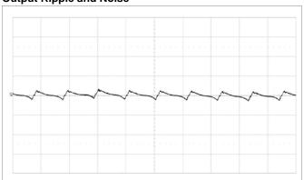
Fundamental output voltage ripple at V<sub>I</sub> = 12 V,I<sub>O</sub> = 35A,  $C_{OUT}$  = 4 x 330 µF/10 m $\Omega$  + 10 x 100 µF Scale: 10 mV/div, 2 µs/div, 20 MHz bandwidth. See section Output Ripple and Noise.
