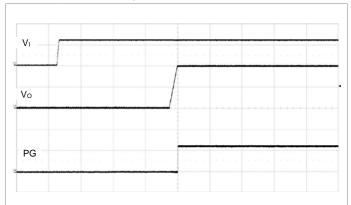
Output enabled by applying V<sub>I</sub>. V<sub>I</sub> = 12 V, I<sub>O</sub> = 80 A. TON\_DELAY = TON\_RISE = 5 ms, POWER\_GOOD\_DELAY = 1 ms. USER\_CONFIG = 0x1084 (page0) / 0x10A4 (page1) (default). Scale from top: 10, 0.5, 2 V/div, 20 ms/div.
