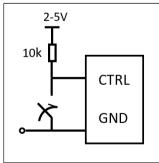
The product is equipped with remote control function. The CTRL pin polarity can be configured active high or active low using PMBus command ON\_OFF\_CONFIG. In active high (positive) mode, CTRL pin requires a pullup resistor to a DC supply to turn on the module. Turn off is achieved by connecting the CTRL pin to GND. And active low (negative) vice versa.
