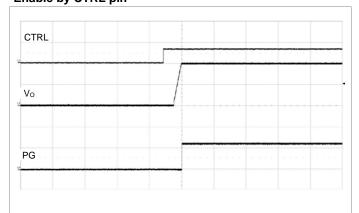
Output enabled by CTRL pin.  $V_1$  = 12 V,  $I_0$  = 80 A. TON\_DELAY = TON\_RISE = 5 ms, POWER\_GOOD\_DELAY = 1 ms. Scale from top: 5, 0.5, 2 V/div, 20 ms/div.
