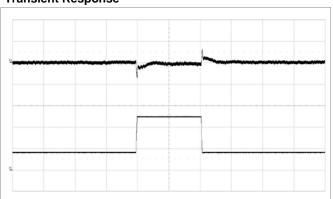
Output voltage response to load current step change (25%-75%-25%) at  $V_{\rm I}$  = 12 V,  $C_{\rm OUT}$  = 8 x 330 µF/10 m $\Omega$  + 20 x 100 µF, di/dt = 2 A/µs, ACSR Gian=219 and ASCR Residual=82.
