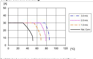
Available load current vs. ambient air temperature and airflow at  $V_{\rm l}$  = 12 V. The other output is enabled at full load, the output voltage is set as 3.3 V.
