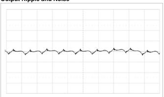
Fundamental output voltage ripple at V<sub>I</sub> = 12 V, I<sub>O</sub> = 30 A, C<sub>OUT</sub> = 4 x 330 µF/10 m $\Omega$  + 10 x 100 µF Scale: 10 mV/div, 2 µs/div, 20 MHz bandwidth. See section Output Ripple and Noise.
