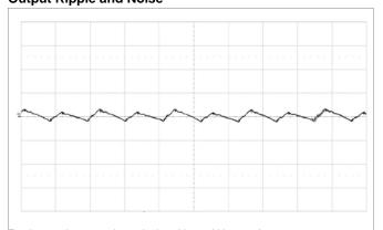
Fundamental output voltage ripple at V<sub>I</sub> = 12 V,I<sub>O</sub> = 70 A, C<sub>OUT</sub> = 8 x 330  $\mu$ F/10 m $\Omega$  + 20 x 100  $\mu$ F Scale: 10 mV/div, 1  $\mu$ s/div, 20 MHz bandwidth. See section Output Ripple and Noise.
