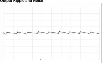
Fundamental output voltage ripple at V<sub>I</sub> = 12 V, I<sub>O</sub> = 40 A,  $C_{OUT}$  = 4 x 330  $\mu$ F/10 m $\Omega$  + 10 x 100  $\mu$ F Scale: 10 mV/div, 2 µs/div, 20 MHz bandwidth. See section Output Ripple and Noise.
