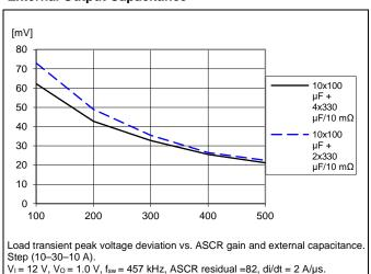
Siep (10–30–10 A).  $V_1$  = 12 V,  $V_0$  = 1.0 V,  $f_{sw}$  = 457 kHz, ASCR residual =82, di/dt = 2 A/ $\mu$ s. ASCR gain changed by PMBus command ASCR\_CONFIG.
