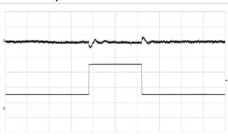
Output voltage response to load current step change (25%-75%-25%) at  $V_{\rm I}$  = 12 V,  $C_{\rm OUT}$  = 8 x 330  $\mu$ F/10 m $\Omega$  + 20 x 100  $\mu$ F, di/dt = 2 A/ $\mu$ s, ACSR Gian=100 and ASCR Residual=82.
