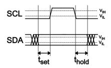
Setup and hold times timing diagram.
