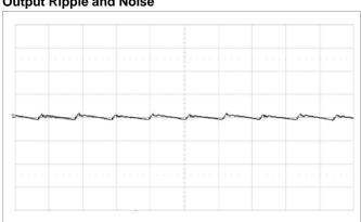
Fundamental output voltage ripple at  $V_1 = 12 \text{ V}$ ,  $I_0 = 80 \text{ A}$ ,  $C_{OUT} = 8 \times 330 \ \mu F / 10 \ m\Omega + 20 \times 100 \ \mu F$ Scale: 10 mV/div, 1 µs/div, 20 MHz bandwidth. See section Output Ripple and Noise.
