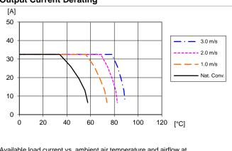
Available load current vs. ambient air temperature and airflow at  $V_{\rm l}$  = 12 V. The other output is enabled at full load, the output voltage is set as 2.5 V.
