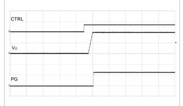
Output enabled by CTRL pin.  $V_l$  = 12 V,  $l_0$  = 40 A. TON\_DELAY = TON\_RISE = 5 ms, POWER\_GOOD\_DELAY = 1 ms. Scale from top: 5, 0.5, 2 V/div, 20 ms/div.
