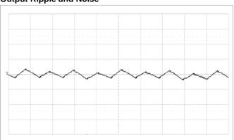
Fundamental output voltage ripple at V<sub>I</sub> = 12 V, I<sub>O</sub> = 65 A, C<sub>OUT</sub> = 8 x 330  $\mu$ F/10 m $\Omega$  + 20 x 100  $\mu$ F Scale: 10 mV/div, 1 µs/div, 20 MHz bandwidth. See section Output Ripple and Noise.
