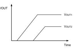
Illustration of Output Voltage Sequencing.
