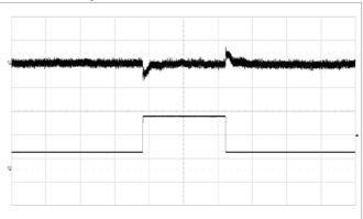
Output voltage response to load current step change (25%–75%–25%) at V<sub>I</sub> = 12 V, C<sub>OUT</sub> = 4 x 330  $\mu$ F/10 m $\Omega$  + 10 x 100  $\mu$ F, di/dt = 2 A/ $\mu$ s, ACSR Gian=219 and ASCR Residual=82. Scale from top: 50 mV/div, 10 A/div, 1 ms/div.
