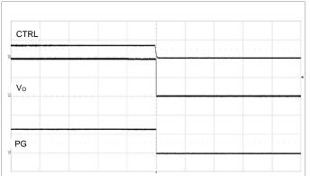
Output disabled by CTRL pin.  $V_I$  = 12 V,  $I_O$  = 40 A. Scale from top: 5, 0.5, 2 V/div, 20 ms/div.
