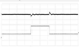
Output voltage response to load current step change (25%–75%–25%) at  $V_1$  = 12 V,  $C_{OUT}$  = 8 x 330  $\mu$ F/10 m $\Omega$  + 20 x 100  $\mu$ F, di/dt = 2 A/ $\mu$ s, ACSR Gian=219 and ASCR Residual=82.
