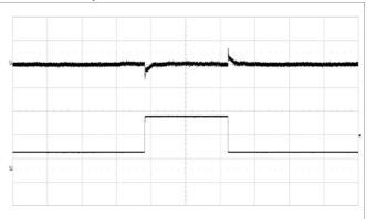
Output voltage response to load current step change (25%–75%–25%) at  $V_{I}$  = 12 V,  $C_{OUT}$  = 4 x 330  $\mu$ F/10  $m\Omega$  + 10 x 100  $\mu$ F, di/dt = 2 A/ $\mu$ s, ACSR Gian=219 and ASCR Residual=82. Scale from top: 50 mV/div, 10 A/div, 1 ms/div.
