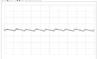
Fundamental output voltage ripple at V<sub>I</sub> = 12 V, I<sub>O</sub> = 80 A, C<sub>OUT</sub> = 8 x 330  $\mu$ F/10 m $\Omega$  + 20 x 100  $\mu$ F Scale: 10 mV/div, 1  $\mu$ S/div, 20 MHz bandwidth. See section Output Ripple and Noise.
