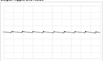
Fundamental output voltage ripple at V<sub>I</sub> = 12 V, I<sub>O</sub> = 40 A, C<sub>OUT</sub> = 4 x 330  $\mu$ F/10 m $\Omega$  + 10 x 100  $\mu$ F Scale: 10 mV/div, 2  $\mu$ S/div, 20 MHz bandwidth. See section Output Ripple and Noise.
