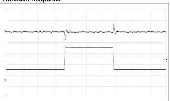
Output voltage response to load current step change (25%-75%-25%) at  $V_1 = 12 \text{ V}$ ,  $C_{OUT} = 4 \times 330 \ \mu\text{F}/10 \ \text{m}\Omega + 10 \times 100 \ \mu\text{F}$ ,  $di/dt = 2 \ \text{A}/\mu\text{s}$ , ACSR Gian=219 and ASCR Residual=82.
