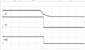
Output disabled by removing V<sub>I</sub>.  $V_I$  = 12 V,  $I_O$  = 40 A. Scale from top: 10, 0.5, 2 V/div, 20 ms/div.
