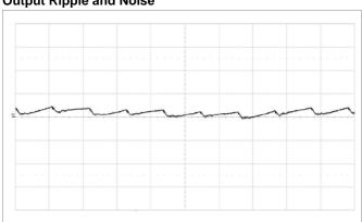
Fundamental output voltage ripple at V<sub>I</sub> = 12 V,I<sub>O</sub> = 40 A,  $C_{OUT} = 8 \times 330 \ \mu F / 10 \ m\Omega + 20 \times 100 \ \mu F$ Scale: 10 mV/div, 1 µs/div, 20 MHz bandwidth. See section Output Ripple and Noise.
