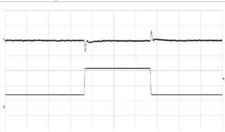
Output voltage response to load current step change (25%–75%–25%) at  $V_{I}$  = 12 V,  $C_{OUT}$  = 4 x 330  $\mu F/10$  m $\Omega$  + 10 x 100  $\mu F,$  di/dt = 2 A/ $\mu s,$  ACSR Gian=219 and ASCR Residual=82. Scale from top: 50 mV/div, 10 A/div, 200  $\mu s/div.$
