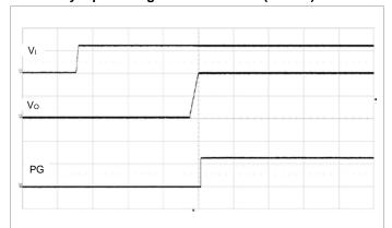
Output enabled by applying  $V_i$ .  $V_i$  = 12  $V_i$   $I_0$  = 40 A. TON\_DELAY = TON\_RISE = 5 ms, POWER\_GOOD\_DELAY = 1 ms. USER\_CONFIG = 0x1084 (page0) / 0x10A4 (page1) (default). Scale from top: 10, 0.5, 2 V/div, 20 ms/div.
