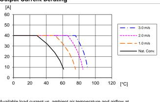
Available load current vs. ambient air temperature and airflow at
