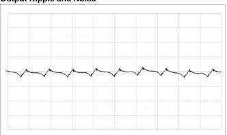
Fundamental output voltage ripple at V<sub>I</sub> = 12 V, I<sub>O</sub> = 32.5 A,  $C_{OUT}$  = 4 x 330 µF/10 m $\Omega$  + 10 x 100 µF Scale: 10 mV/div, 2 µs/div, 20 MHz bandwidth. See section Output Ripple and Noise.
