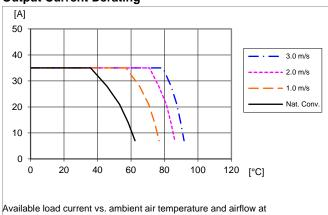
The other output is enabled at full load, the output voltage is set as 1.8 V.
