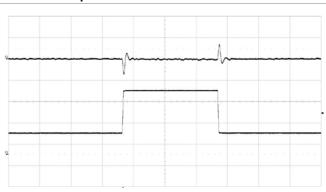
Output voltage response to load current step change (25%–75%–25%) at  $V_1$  = 12 V,  $C_{OUT}$  = 4 x 330  $\mu$ F/10 m $\Omega$  + 10 x 100  $\mu$ F, di/dt = 2 A/ $\mu$ s, ACSR Gian=219 and ASCR Residual=82.
