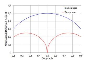
The input ripple RMS current in a buck converter can be estimated to
