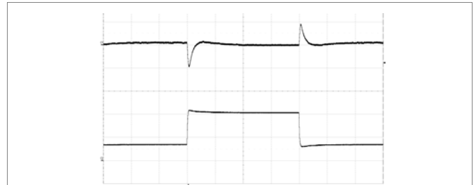
Output disabled by removing V_i at: T_{P1} = +25^{\circ}\text{C} , V_i = 48\text{ V} , I_o = 3\text{ A} electronic load. Top trace: output voltage (2 V/div.). Bottom trace: input voltage (20 V/div.). Time scale: (1 ms/div.).
