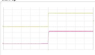
Start-up enabled by connecting V<sub>I</sub> at:  $T_{P1} = +25^{\circ}C, V_{I} = 110 V,$ lo = 2.5 A resistive load.
