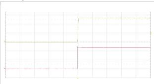
Start-up enabled by connecting V<sub>I</sub> at:  $T_{P1} = +25^{\circ}C, V_{I} = 110 V,$ lo = 0.555 A resistive load.
