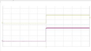
Start-up enabled by connecting V<sub>I</sub> at:  $T_{P1} = +25^{\circ}C, V_{I} = 110 V,$ lo = 2 A resistive load.
