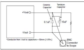
Output ripple and noise test setup
