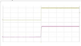
Start-up enabled by connecting V<sub>I</sub> at:  $T_{P1} = +25^{\circ}C, V_{I} = 110 V,$ lo = 6 A resistive load.
