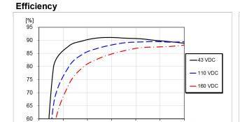
Efficiency vs. load current and input voltage at +25°C.
