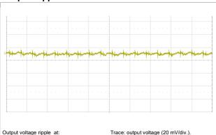
Output voltage ripple at: T<sub>P1</sub> = +25°C, VI = 110 V, Io = 6 A resistive load
