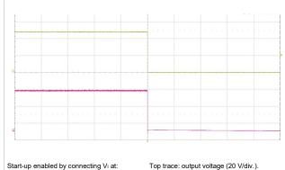
T<sub>P1</sub> = +25°C, V<sub>I</sub> = 110 V, Io = 0.625 A resistive load. Bottom trace: input voltage (50 V/div.). Time scale: (200 ms/div.).
