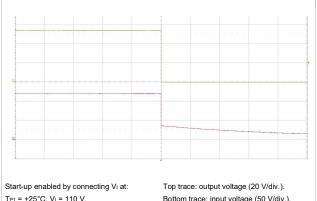
T<sub>P1</sub> = +25°C, V<sub>I</sub> = 110 V, Io = 0.555 A resistive load. Bottom trace: input voltage (50 V/div.). Time scale: (200 ms/div.).
