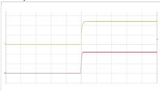
Start-up enabled by connecting V<sub>I</sub> at:  $T_{P1} = +25^{\circ}C, V_{I} = 110 V,$ lo = 1.25 A resistive load.
