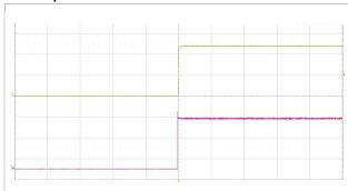
Start-up enabled by connecting V<sub>I</sub> at:  $T_{P1} = +25^{\circ}C, V_{I} = 110 V,$ lo = 0.625 A resistive load.
