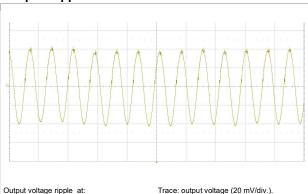
T<sub>P1</sub> = +25°C, VI = 110 V, lo = 0.625 A resistive load. Time scale: (5 µs/div.). 20MHz bandwidth
