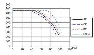
Available power at given ambient air temperature vs. thermal option at V<sub>I</sub> = 54 V. See Thermal Consideration section.
