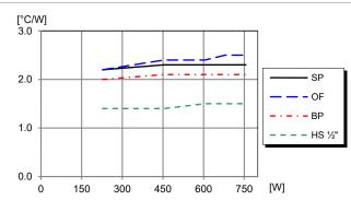
Thermal resistance at given power vs. thermal option at given airspeed measured at the converter. Tested in wind tunnel with airflow and test conditions as per the Thermal consideration section.
