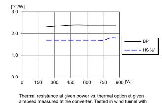
airspeed measured at the converter. Tested in wind tunnel with airflow and test conditions as per the Thermal consideration section.
