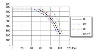
Available power at given ambient air temperature vs. thermal option at
