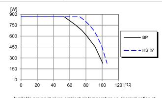
Available power at given ambient air temperature vs. thermal option at  $V_1 = 54 \text{ V}$ . See Thermal Consideration section.
