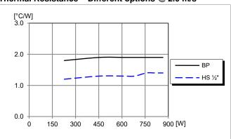
Thermal resistance at given power vs. thermal option at given airspeed measured at the converter. Tested in wind tunnel with airflow and test conditions as per the Thermal consideration section.  $V_1 = 54 V.$
