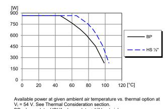
BP = base plate, HS½" = base plate + ½" heat sink.
