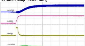
Blue line – output voltage 1 V/div Red line – input voltage change 54-44-72 V, 20 V/div Yellow line –input current supplied from the HU- capacitor, 50 A/div Green line – output current, 50 A/div 2 ms/div
