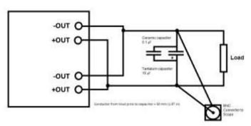
Output ripple and noise test setup
