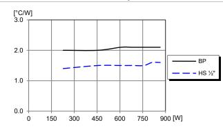
Thermal resistance at given power vs. thermal option at given airspeed measured at the converter. Tested in wind tunnel with airflow and test conditions as per the Thermal consideration section.  $V_1 = 54 V.$
