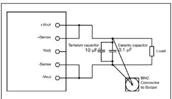
Output ripple and noise test setup
