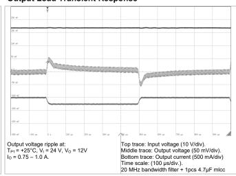
Output voltage ripple at:  $T_{P1}$  = +25°C,  $V_1$  = 24 V,  $V_0$  = 12V  $I_0$  = 1 A resistive load.
