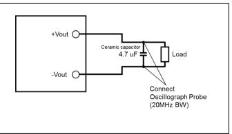
Output ripple and noise test setup
