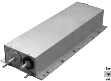
The 4000W LSM power module is a high voltage liquid cooled DC-DC converter which steps down 400V and provides 24V output, common in hybrid and electric vehicle applications. The output voltage is electrically isolated from the input voltage and suits the conventional 24V accessories and HVAC system requirements of industrial and ecofriendly vehicles.
