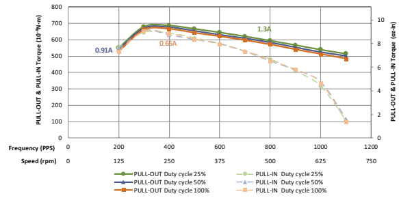
42PM096L-00701 (7Ω) Rated Voltage 24V Constant Current Bipolar Full-Step
