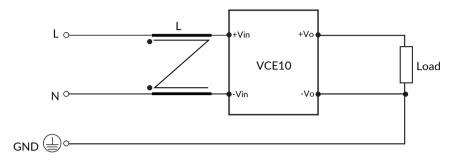
Suggested value - L: 20mH, 500mA common mode choke such as Würth Elektronik 744821120.
