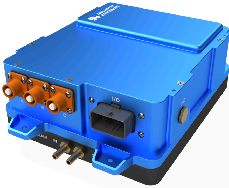
Figure 1. The SOLO PRO 400-160 — a complete 150–450 VDC, 160 A liquid-cooled motor drive. The front face carries the three motor outputs A, B and C, the 48-pin I/O connector and the coolant inlet and outlet. The sealed USB port is on the right face.
