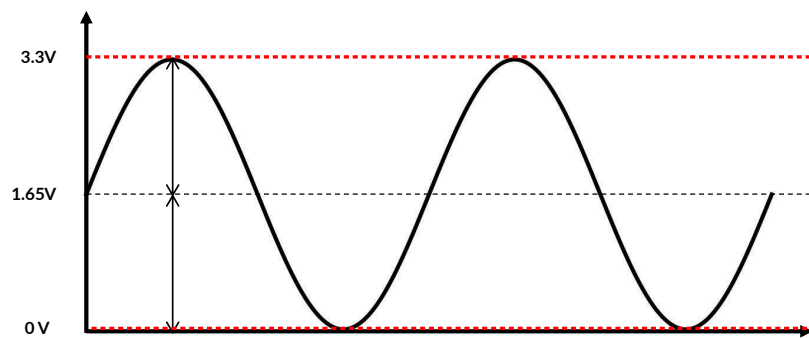
Figure 33. Sin/Cos input to the DSP: sine and cosine centred on 1.65 V with the swing kept within the 0–3.3 V ADC range. The full range need not be used (e.g. 0.5–2.8 V is acceptable) as long as the signals stay centred on 1.65 V. A larger amplitude yields finer interpolation resolution.
