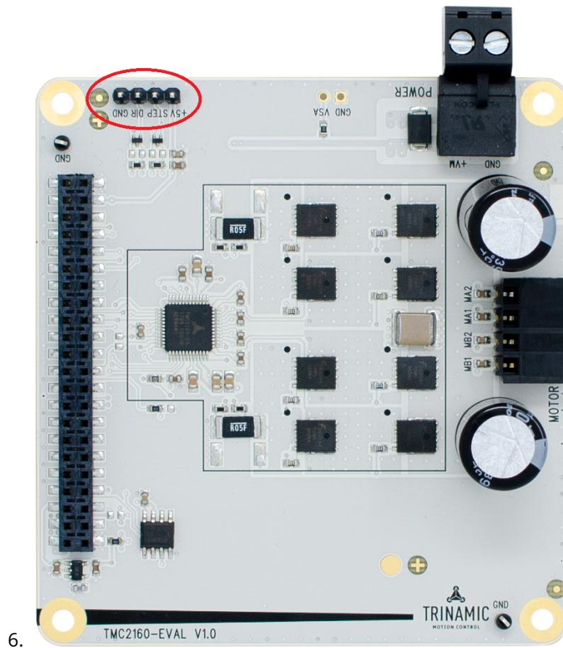
Figure 3: Pin Headers on the TMC2160-EVAL
