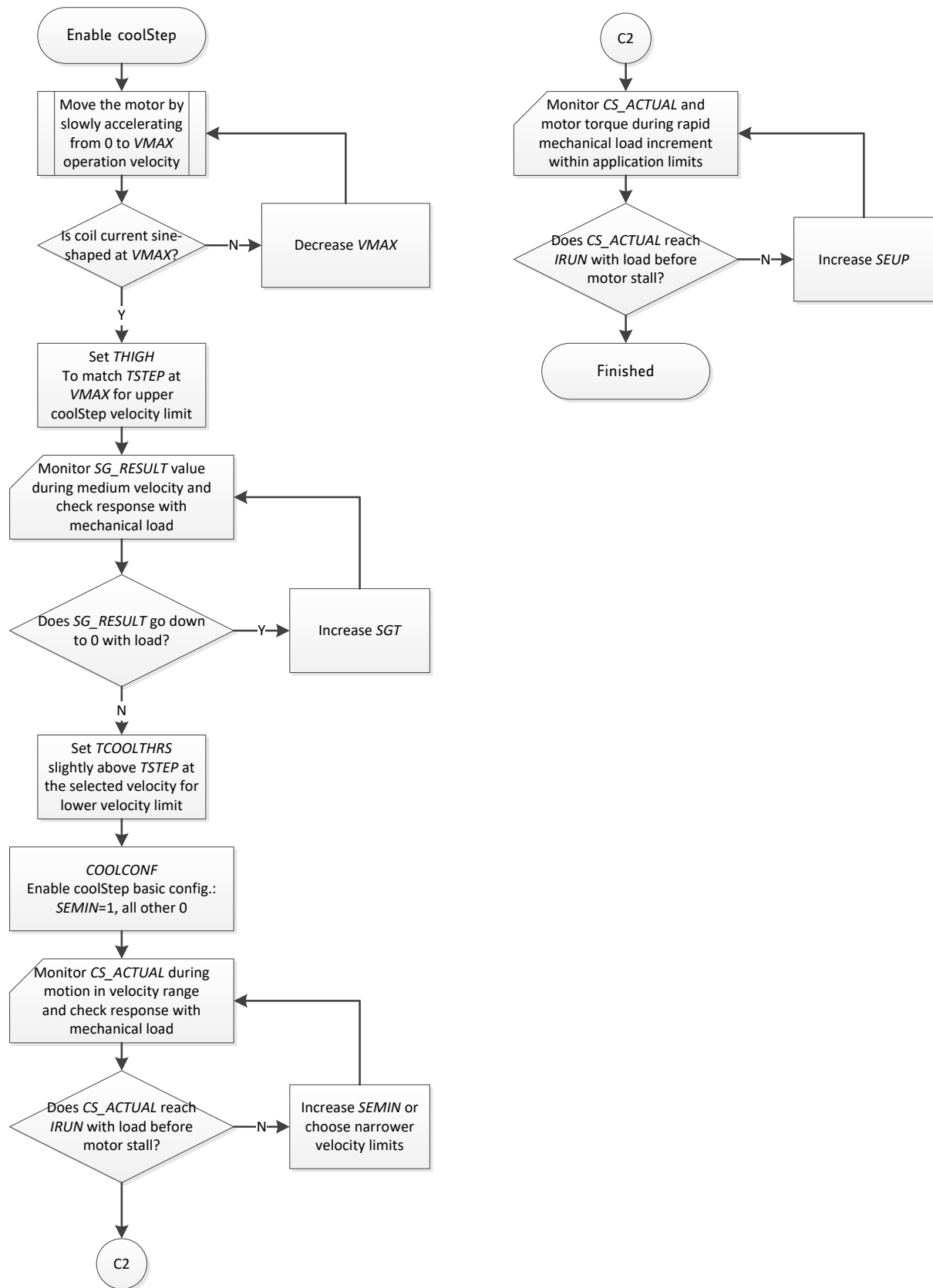
Figure 22.4 Enabling coolStep (only in combination with spreadCycle)
