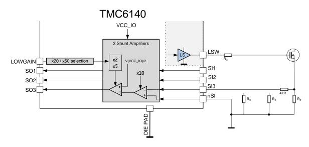
Figure 12: Shunt Amplifier setup for phase W
