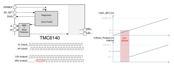
*Figure 10: Impact of SH\_SET configuration.*
