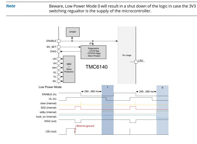
Figure 8: Illustration of the activation of the two available Low Power Modes
