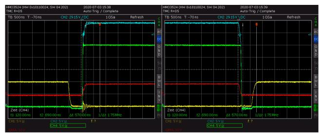
Figure 6: Ringing of output (green) and gate voltages (yellow, blue) with DRV\_STRONG=0
