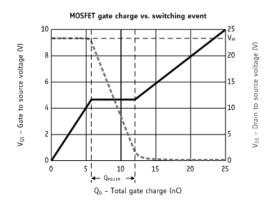
Figure 4: Miller charge determines switching slope
