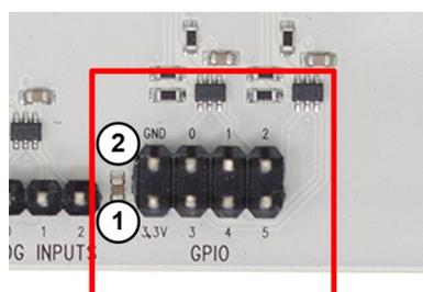
Figure 18: TMCM-1617-BB GPIO Header
