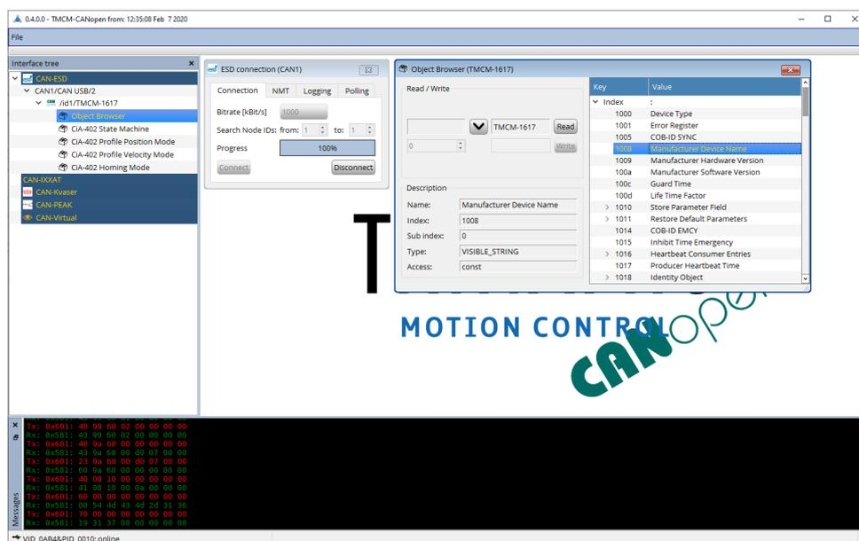
Figure 6: The TMCM-CANopen Tool with TMCM-1617 successfully connected
