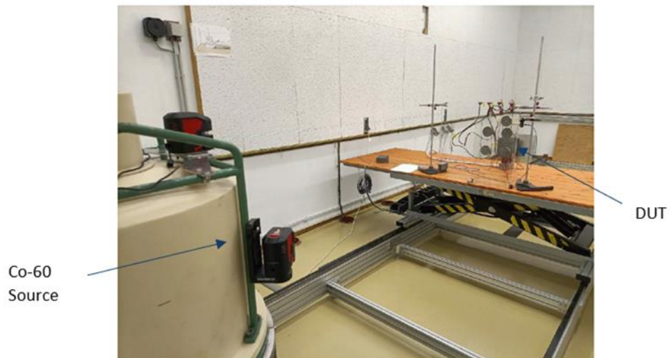
Figure 3 Set up inside the irradiation chamber showing the Co-60 source and devices under test; the rails on the floor enable the holding fixture to be positioned for the desired radiation levels
