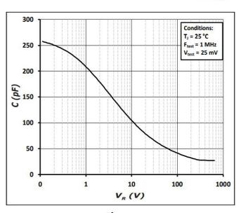
**Figure 6**Capacitace vs. Reverse Voltage
