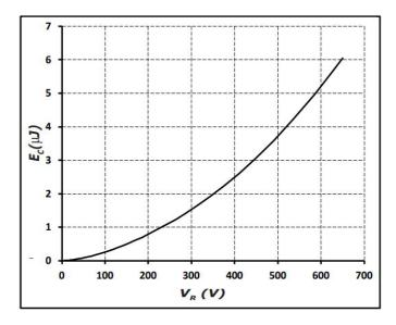
**Figure 7**Capacitance Stored Energy
