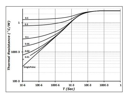
Figure 9 Transient Thermal Impedance
