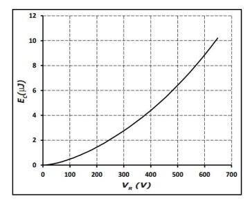
**Figure 7**Capacitance Stored Energy
