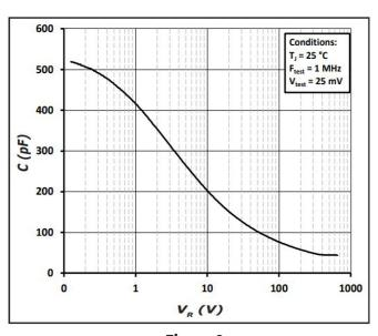
**Figure 6**Capacitace vs. Reverse Voltage
