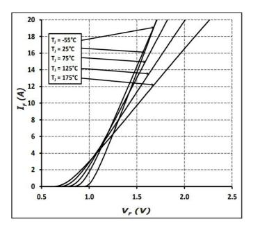
**Figure 1**Forward Characteristics
