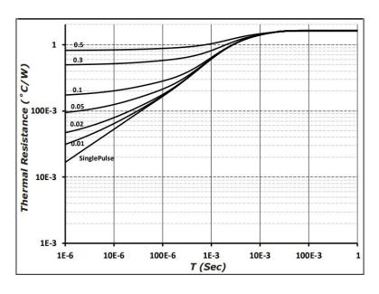
Figure 9 Transient Thermal Impedance
