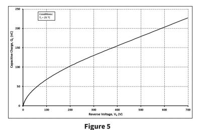
Total Capacitance Charge vs. Reverse Voltage
