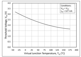
Figure 10. Threshold Voltage vs. Junction Temperature
