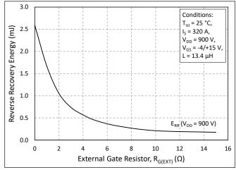
Figure 16. Reverse Recovery Energy vs. External Gate Resistance
