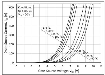
Figure 4. Transfer Characteristic for Various Junction Temperatures
