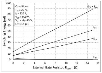
Figure 15. MOSFET Switching Energy vs. External Gate Resistance
