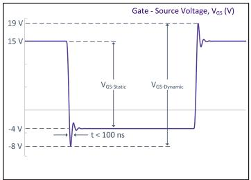
Figure 33.  $V_{GS}$  Transient Definitions
