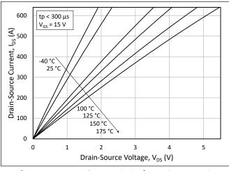
Figure 1. Output Characteristics for Various Junction Temperatures
