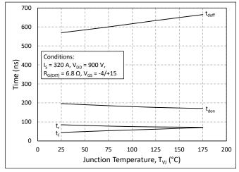
Figure 26. Timing vs. Junction Temperature
