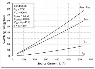
Figure 11. Switching Energy vs. Drain Current ( $V_{DD}$  = 900 V)
