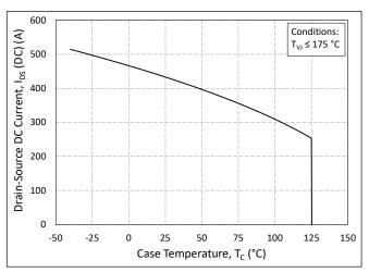
Figure 20. Continuous Drain Current Derating vs. Case Temperature
