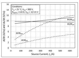
Figure 25. dv/dt and di/dt vs. Source Current
