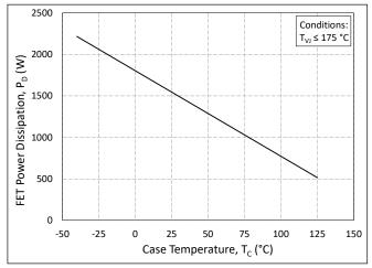
Figure 21. Maximum Power Dissipation Derating vs. Case Temperature
