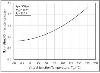
Figure 3. Normalized On-State Resistance vs. Junction Temperature
