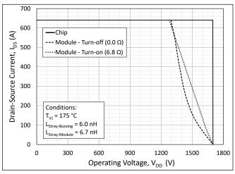
Figure 19. Switching Safe Operating Area
