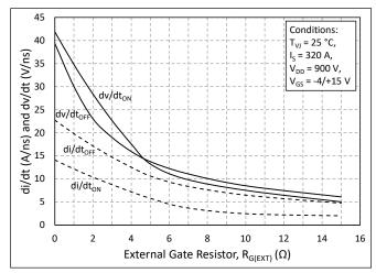
Figure 29. dv/dt and di/dt vs. External Gate Resistance
