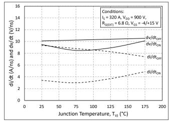
Figure 27. dv/dt and di/dt vs. Junction Temperature
