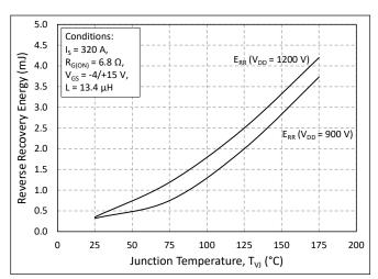
Figure 14. Reverse Recovery Energy vs. Junction Temperature
