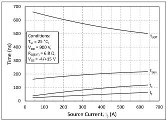
Figure 24. Timing vs. Source Current
