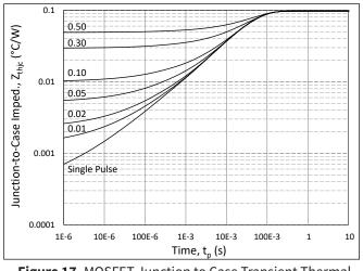
Figure 17. MOSFET Junction to Case Transient Thermal Impedance, Z<sub>th JC</sub> (°C/W)
