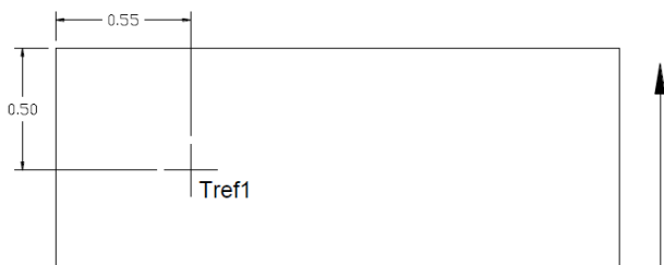
Figure 18. Case ( T_{REF} ) Temperature Measurement Location (top view).
