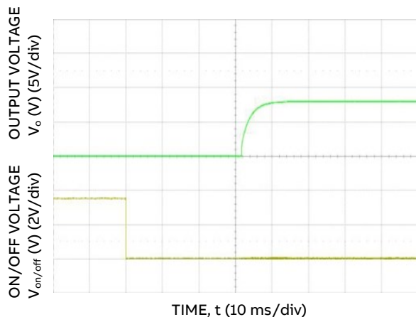
Figure 5. Typical Start-up Using Remote On/Off, negative logic version shown ( V_{in} = 48V , I_o = I_{o,max} ).
