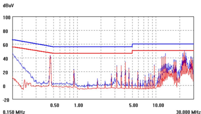
Figure 18. EMC signature using above filter, KHHD010A0.
